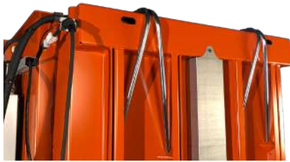
Pipes for easy bale strapping
